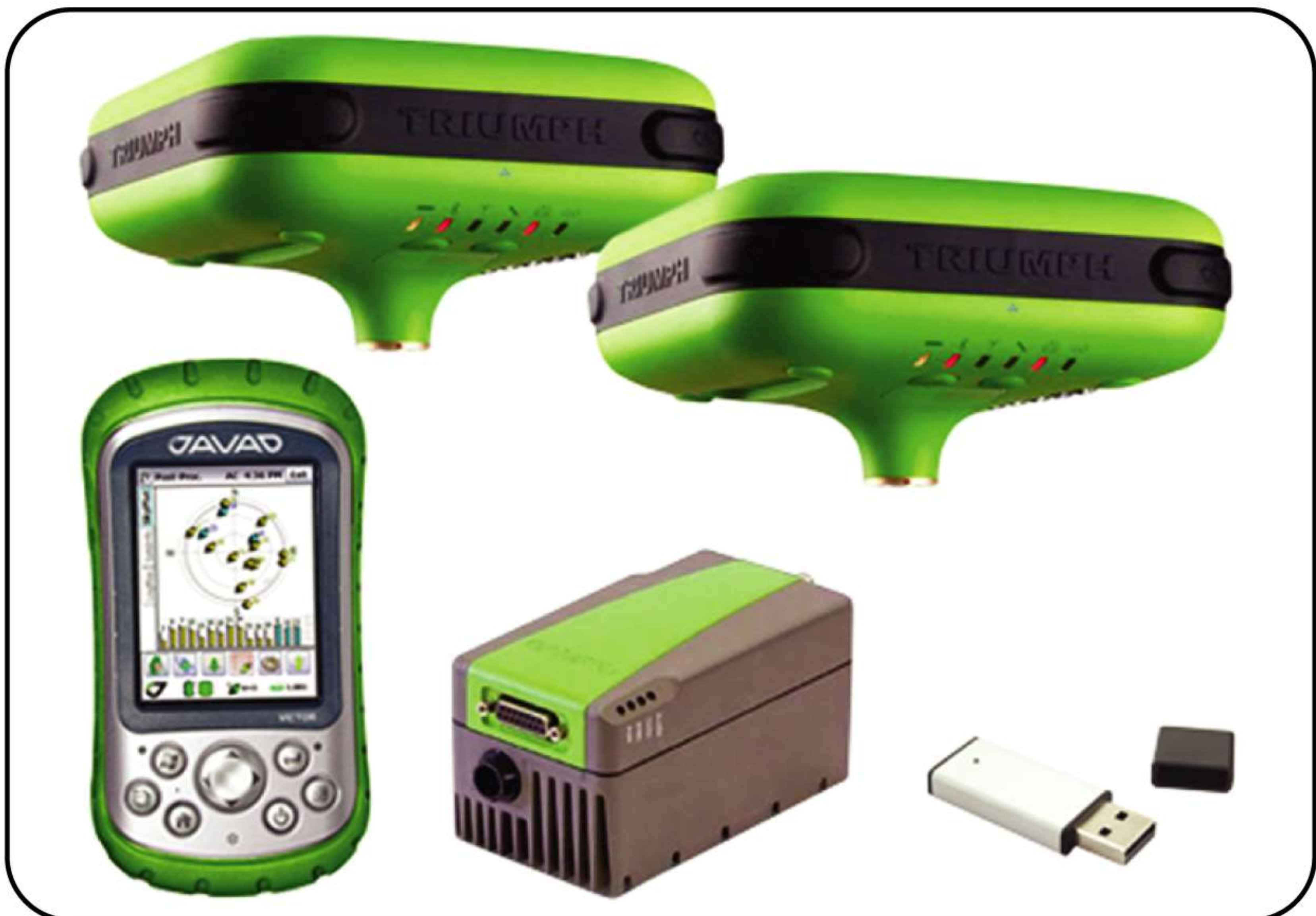
Differential Global Positioning System (DGPS)- JAVAD GNSS
